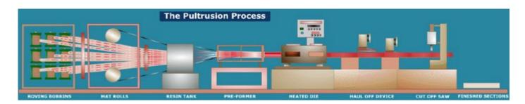
Pultrusion is the process of pulling fiberglass reinforcements such as mats and strands through a proprietary resin and heated die. The result is a specific complex profile that can be cut to any length. This process offers speed and consistency making it the best method for producing high-volume linear fiberglass products that require constant cross sections.
